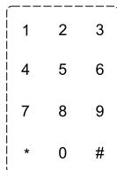
**i Note:** The star key (\*) is assigned the cancel function while the device is being configured and in code lock mode.
