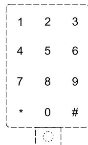
**i Note:** The star key (\*) is assigned the cancel function while the device is being configured and in code lock mode. The hash key (#) is assigned the save function.
