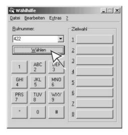
The controlled phone is called. As soon as you pick up the receiver, the destination number dialled (in this example: 422) is called.
