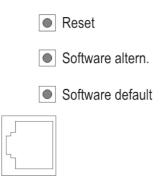
2. Within the space of two seconds, push the **Software altern.** button on the CPU module and hold it.
