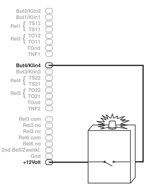
3. Connect the **+12Volt** terminal, for example, to the alarm contact.
