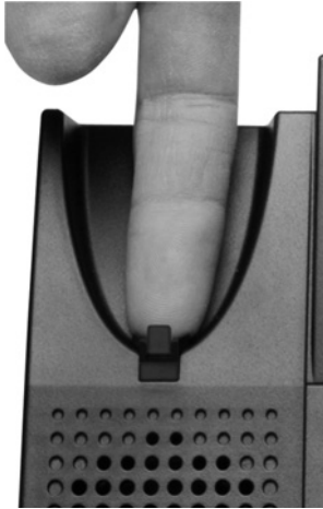
Fig. 12: Pressing down the insert
